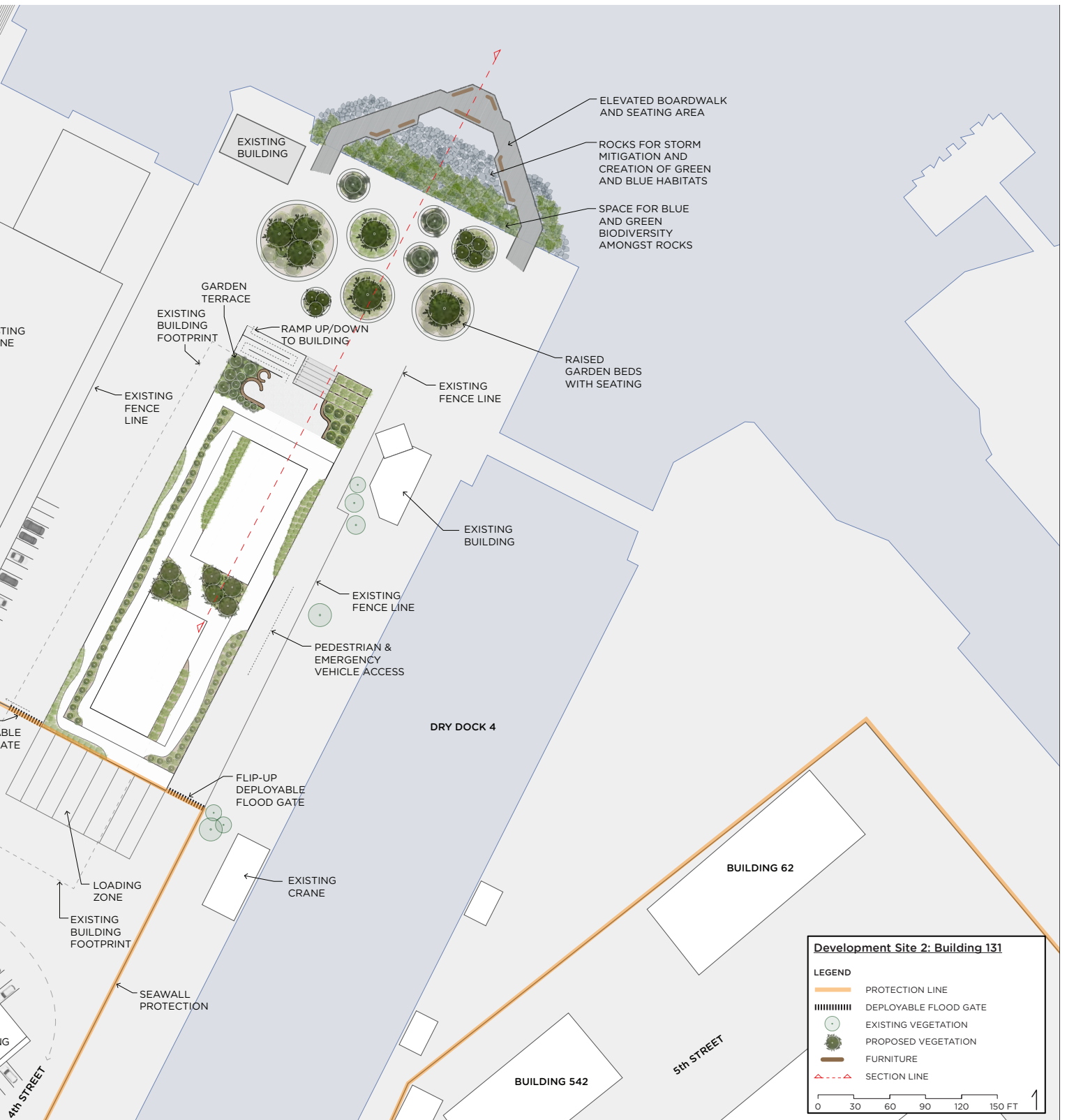
Figure 33. Development Site 2: Building 131 - Site Plan
